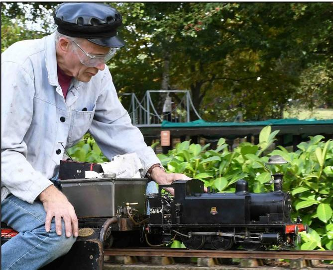
first shown in the *Model Engineer*, finally finishing the model in 1976, the loco has run many miles and been overhauled a number of times since then and was re-tubed in the 1980's.
